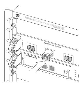
Figure 6: Removing a QSFP+ Module
